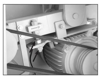
Figure 51. Motor mount nuts.
